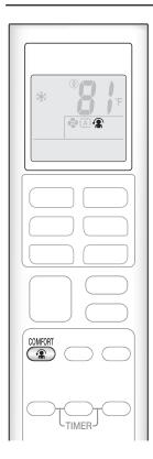
The flow of air will be in the upward direction while in COOL and DRY operation and in the downward direction while in HEAT operation, which will provide a comfortable airflow that will not come in direct contact with people.
