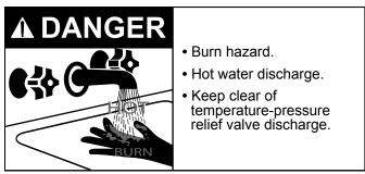
It is recommended that the temperature-pressure relief valve be checked to ensure it is in operating condition at least once a year.
