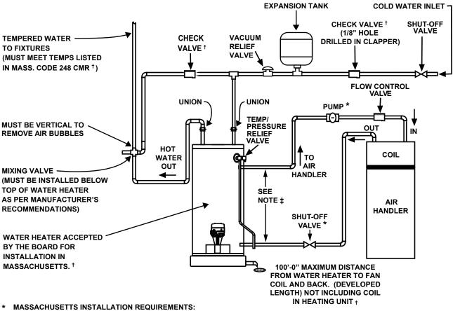
TYPICAL MIXING VALVE INSTALLATION **COMBINATION SPACE HEATING / POTABLE WATER HEATING SYSTEM**
