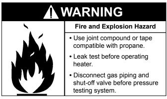
Use pipe joint compound or Teflon tape marked as being resistant to the action of gases.
