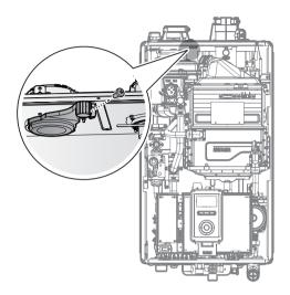
5. Pull the filter out of the boiler.
