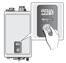
2. Press the Command dial ( ) to select the space heating temperature (IIII). The highlighted section will flash.
