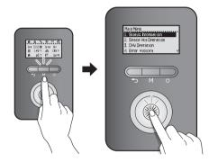
Rotate the Command dial ((3)) to switch between the information items. Press the Command dial ((3)) to select an item and view the information.
