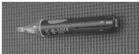
Figure 28 - Use a non-contact circuit tester to check for electrical power.
