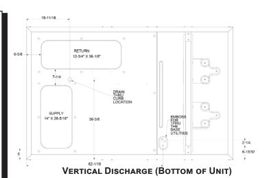
NOTE: REFER TO IOD-7082 INCLUDED IN THE LITERATURE PACK FOR INSTALLING HORIZONTAL DUCT COVERS.
