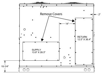
HORIZONTAL DISCHARGE DUCT CONNECTIONS
